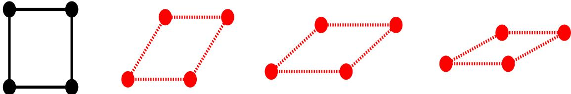
**Telescoping framework:** bars are attached to joints at fixed angles, but are allowed to change in length
